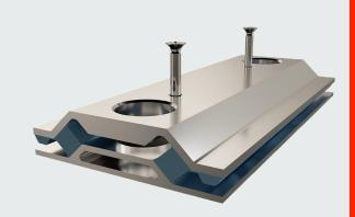
APSOvib® floating floor supports increase passenger's comfort. They are especially developed to absorb external vibrations and compensate for the car body elongation during transit, while keeping weight at a minimum. Our "pick-and place" solution provides with tailor-made interfaces between the floor and the car frame, resulting in additional assembly time savings.
