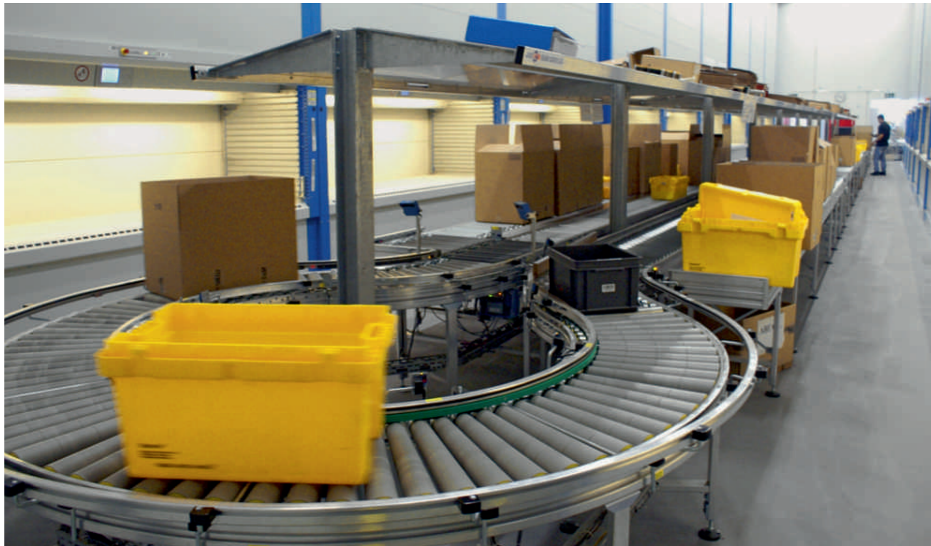
Commercial companies make use of the box conveyor systems of Gilgen Logistics, as do hospitals and libraries. When it comes to the drive of the accumulating roller conveyor and pallet elevator modules, Gilgen Logistics relies on Angst+Pfister's direct current gear motor.
