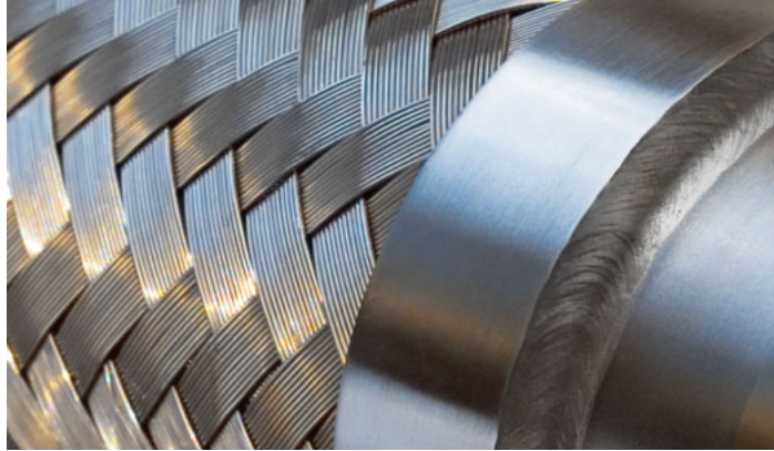
Prototypes, custom fittings, small and very small series and metal hose lines with diameters up to 300 mm are welded manually. High quantities with diameters between 6 and 100 mm are welded mechanically.
