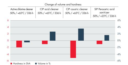
Results of PERTEC® UP EPDM 70.503-04 in different types of CIP/SIP-media, in most challenging concentrations of 50% and over two weeks at +65°C, where appropriate (peracetic acid SIP at room temperature). Very low volume change below 5% and limited hardness changes in the range of -5ShA over this extended time indicate an excellent compound for all applications involving harsh CIP conditions.
