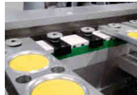
Attachment of capsule carrier plates to the timing belt.
