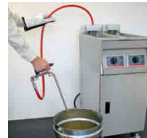
The hot oil is pumped out of the fryer.
