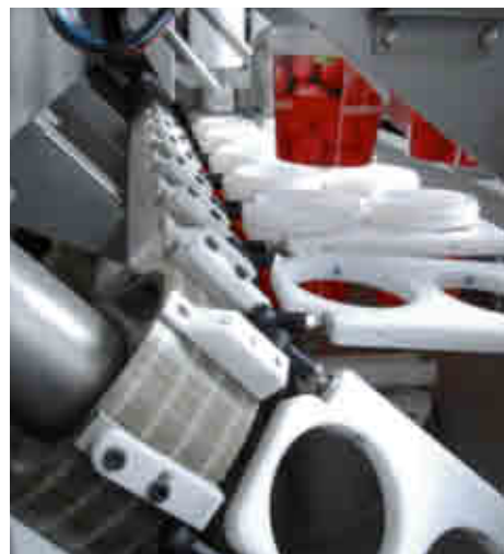
BRECO® ATN timing belt: the profiles can be quickly and easily switched in and out – a difference with far-reaching advantages. The same timing belt can be used to convey a variety of different goods.
