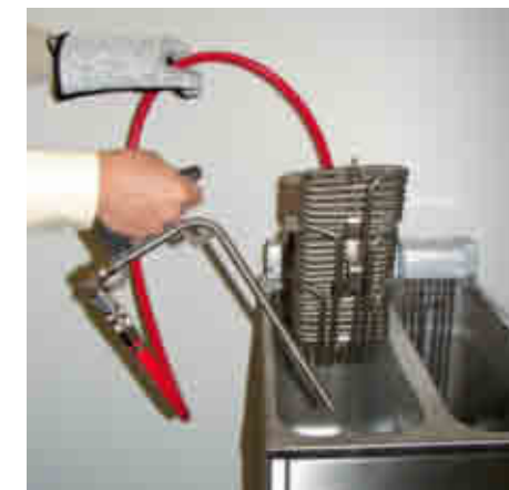
The fryer well is rinsed and filled.
