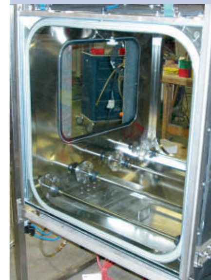
Front view of the infeed opening with the AIRMATIC® sealing system installed around the opening.
