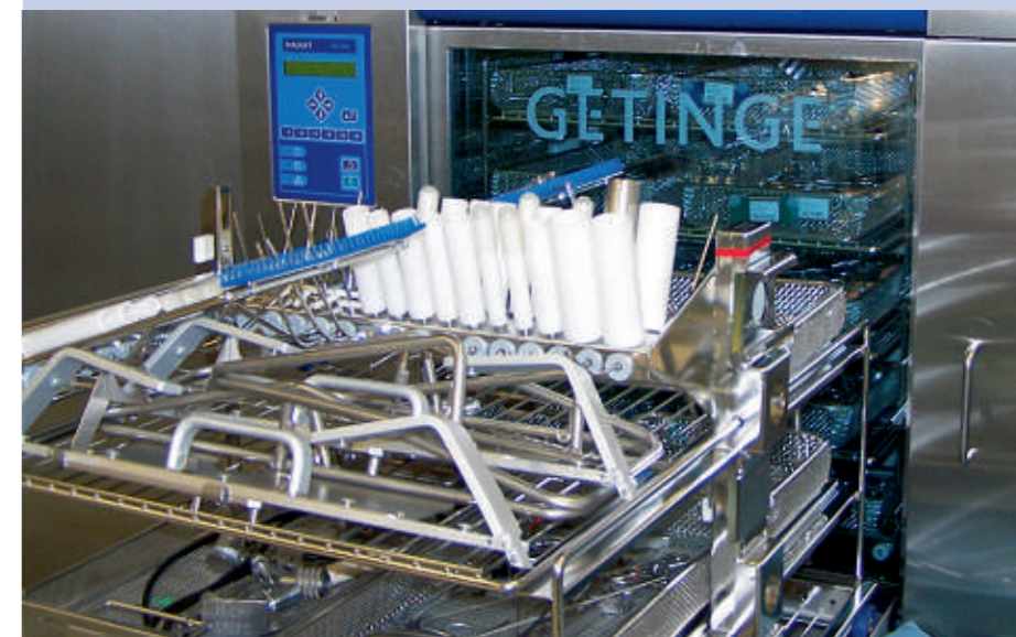
Loaded items ready for washing and disinfecting
