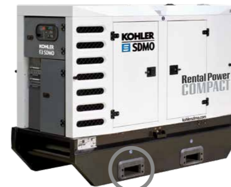
The generators are equipped with protective buffers so that the forklift trucks do not leave any damage when loading and unloading.
